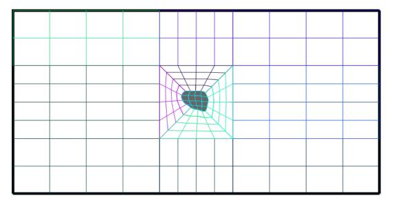
FIG. 3.  $2^{nd}$  order Quadrangular meshing done over the domain shown in the figure 2.
